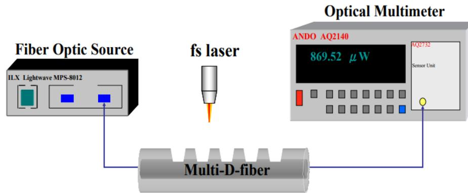
**Figure 2.10: Experimental setup for monitoring the transmission power loss of multi-D-shaped optical fibers during fabrication process**
