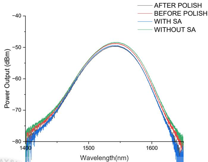
**Figure 4.9: Comparison graph for 1db loss sample by using SMF from 1400nm to 1650nm.**
