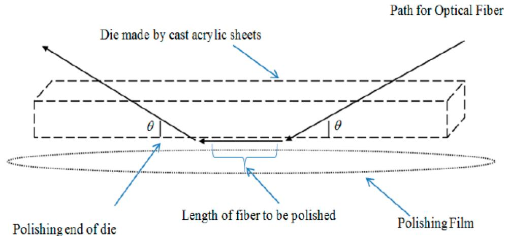
**Figure: 2.9: Ultrapol end and edge polishing system**
