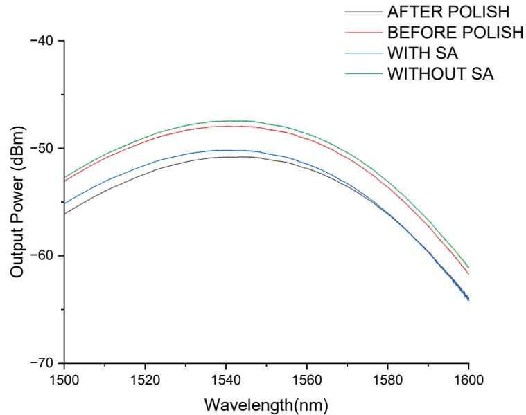
**Figure 4.12: Comparison graph for 2db loss sample by using SMF from 1500nm to 1600nm**
