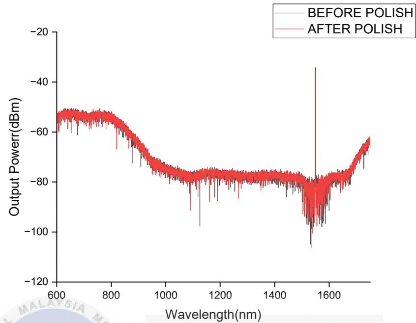
Figure 4.1: Comparison graph of SMF from 600nm to 1750nm
