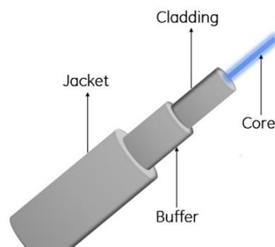
**Figure 2.3: Single-Mode Fiber Construction**
