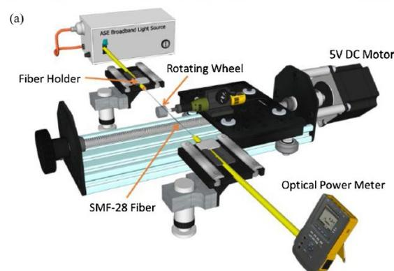
**Figure 2.8: Mechanical polishing technique**
