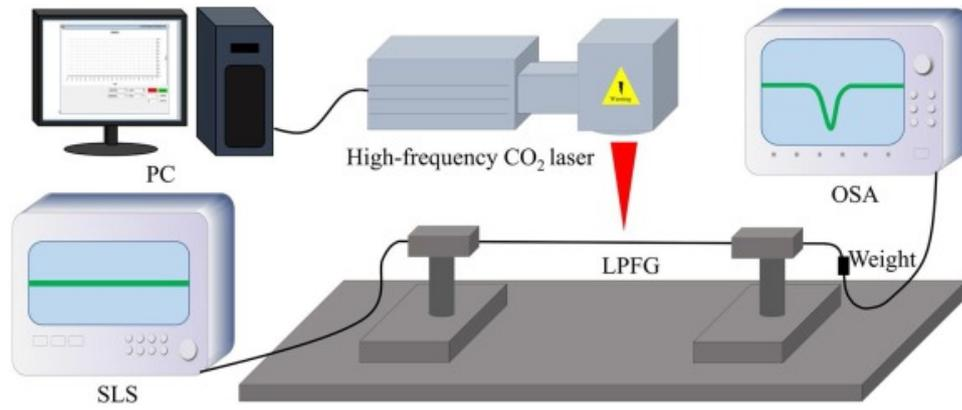
**Figure 2.11: Fabrication method by using CO<sub>2</sub> Laser**
