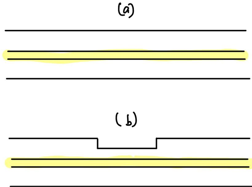
**Figure 3.10: Comparison of normal optical fiber and D-shape optical fiber**
