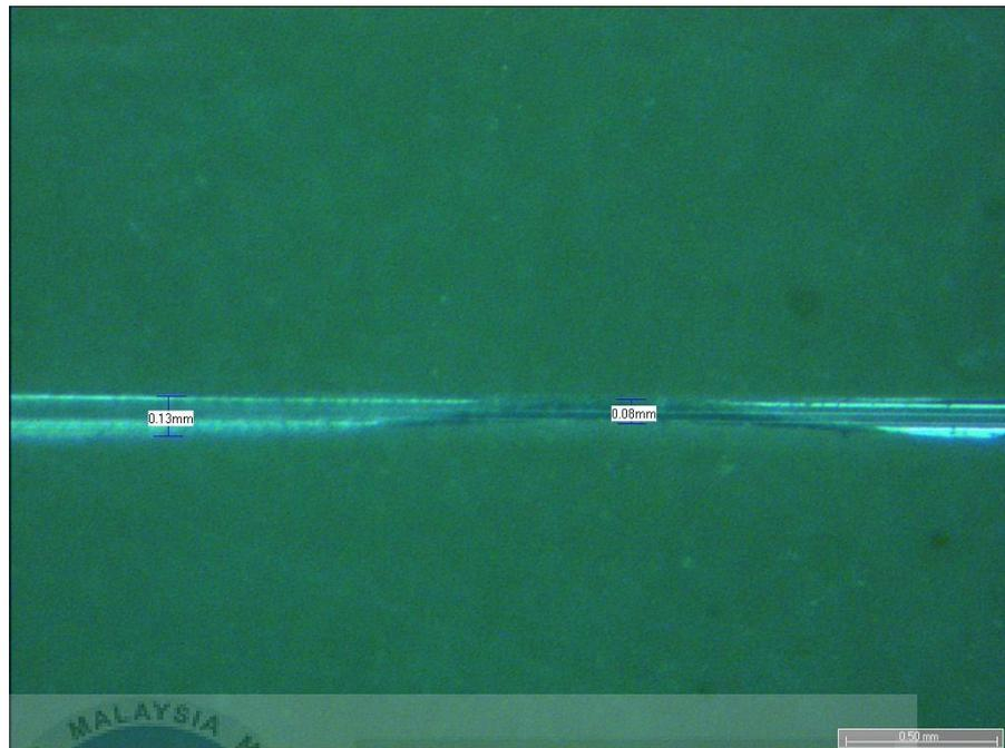
Figure 4.7: Microscopic image of SMF d-shaped optical fiber (1dB loss)
