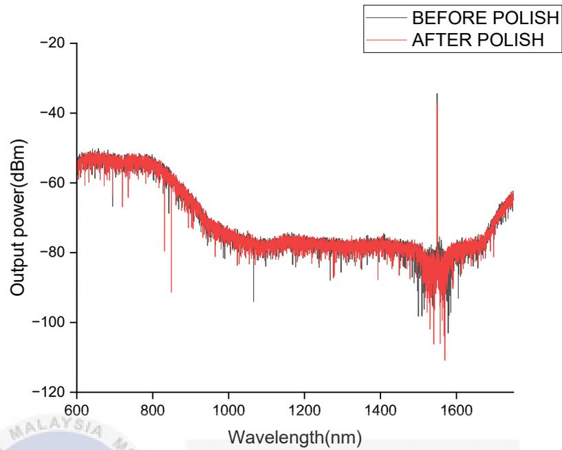
Figure 4.4: Comparison graph of MMF from 600nm to 1750nm
