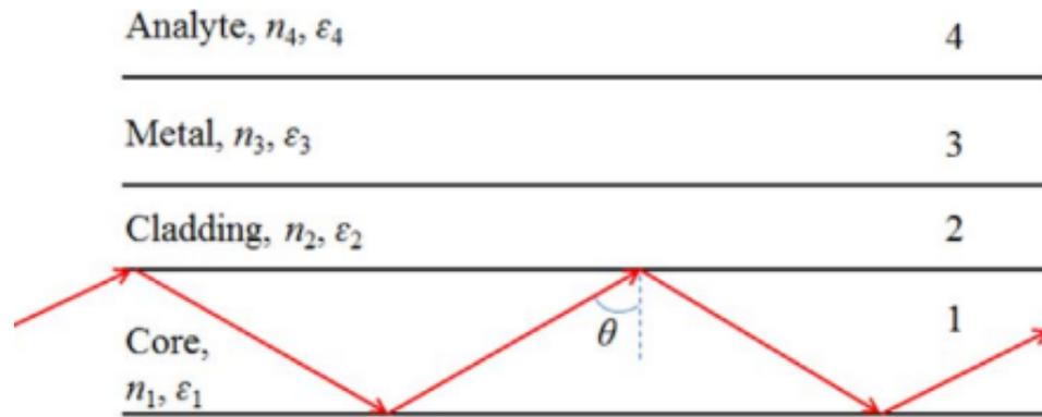
**Figure 2.7: Light transmission model through a D-shaped optical fiber**
