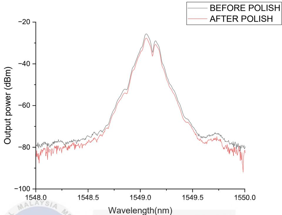
**Figure 4.3: Comparison graph of SMF from 1548nm to 1550nm**
