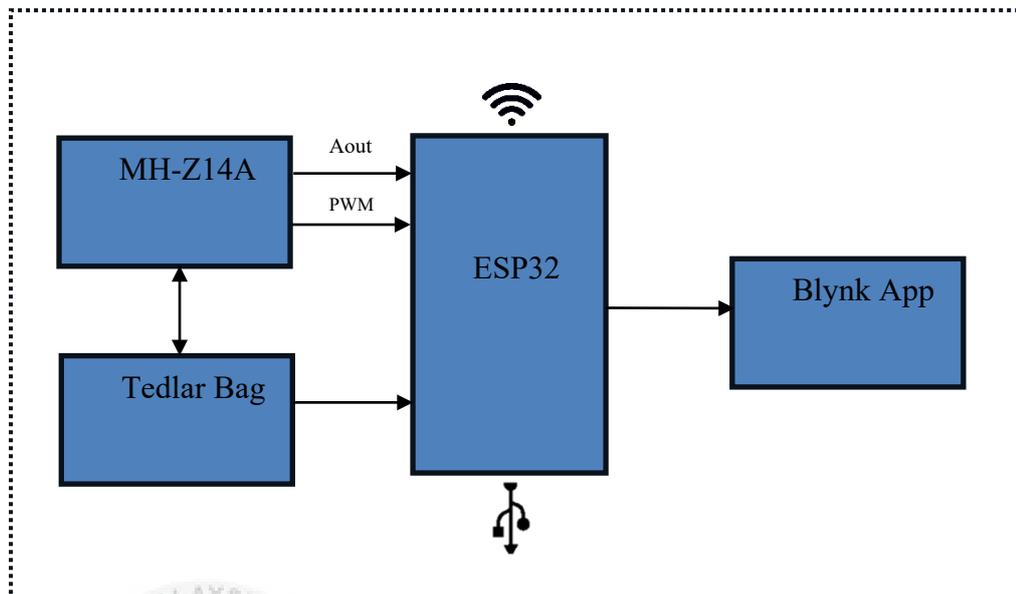
**Figure 3.2: Block Diagram for development of exhaled human breath system.**
