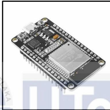
**Figure 3.3: ESP32 Microcontroller.**
