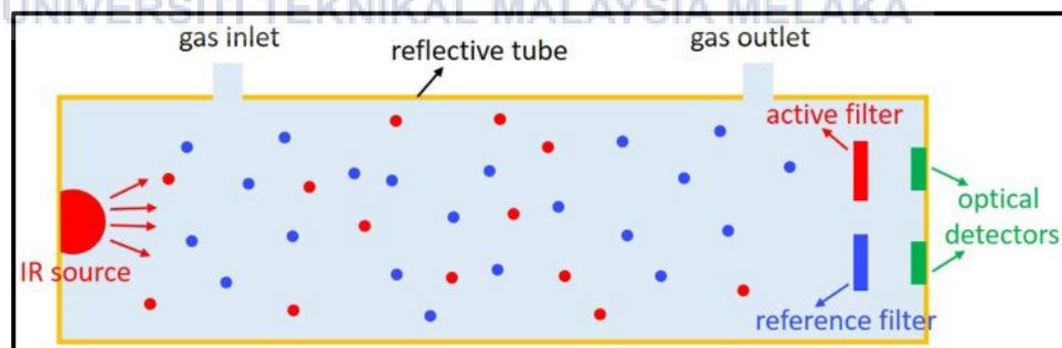
**Figure 2.2: The structure of optical gas sensors [11].**
