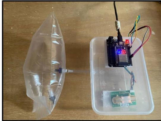
**Figure 3.11: A Prototype Connected with Tedlar Bag.**
