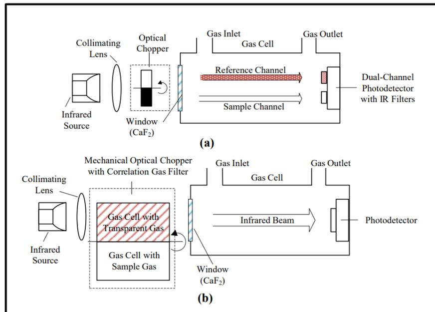
**Figure 2.3: Non-dispersive infrared sensor design: (a) structure of a double beam NDIR sensor, modified from [14] and (b) single-beam non-dispersive infrared sensor design utilizing a correlation gas filter method, adapted from [15].**
