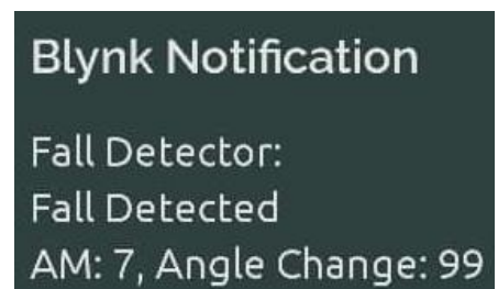
Figure 4.13: AM and angleChange reading from Blynk (Fall Straight)
