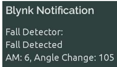
Figure 4.12: AM and angleChange reading from Blynk (Fall Diving)
