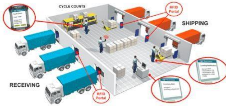
Figure 2.5: Scheme of implementing the RFID technology in a warehouse
