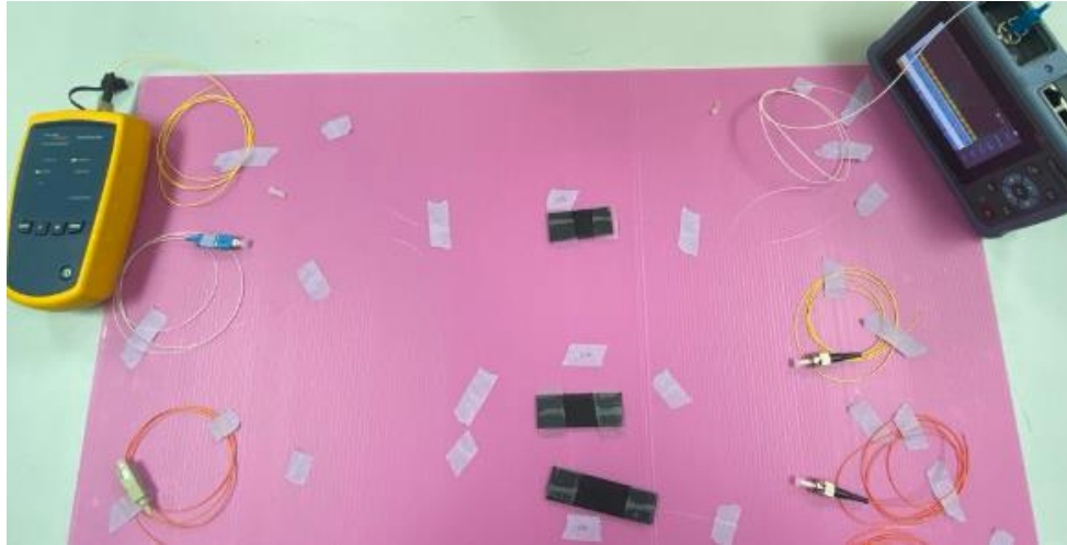
Figure 4.1 Schematic of Optical Fiber Sensor for Glucose Concentration
