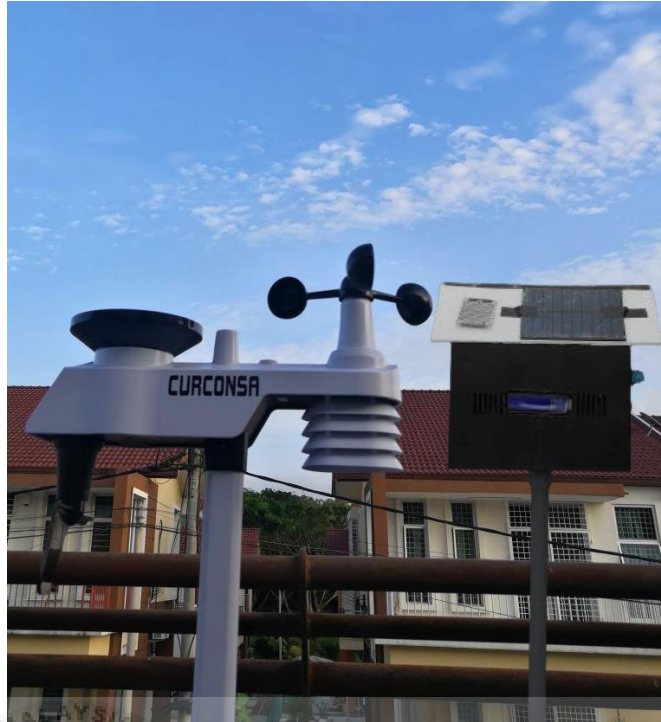
Figure 4.17 Comparison Experimental Weather Station and Commercial Weather Station
