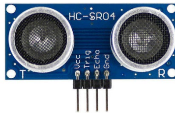
Figure 3.7 Pin of HC-SR04 Ultrasonic sensor[23]
