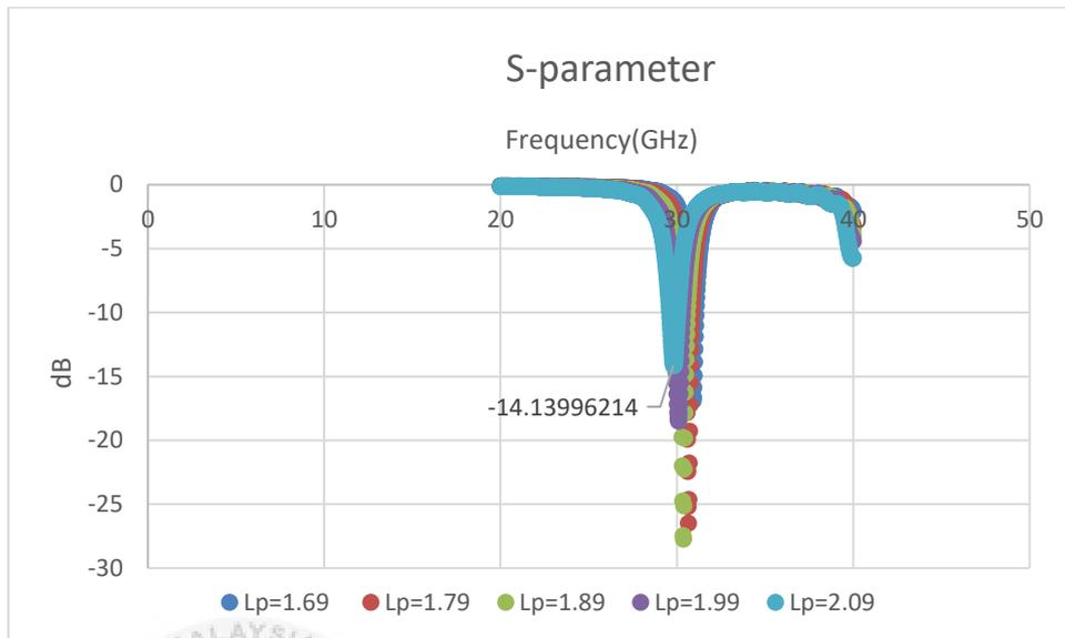
Figure 4.2.1.4 : The S-parameters for FR-4 substrate
