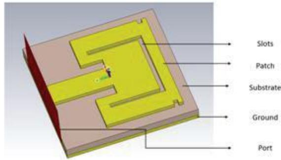
Figure 2.6.1: 3D view of proposed microstrip slotted patch antenna in CST
