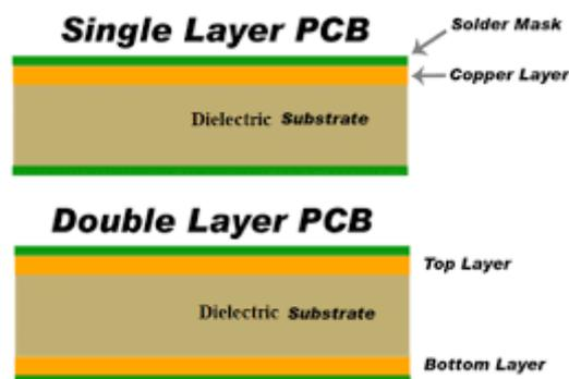
Figure 2.5.3.1: Example of dielectric substrate
