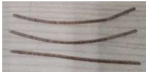
Figure 3.23 The cut up filament after being in the oven for an hour.
