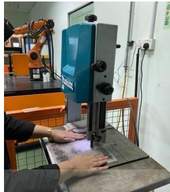
Figure 3.13 The hotpressed composite being cut into half for the crushed machine.
