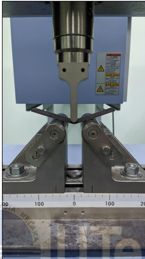
Figure 3.4 Precision universal tester machine (3-Point Bending Test)
