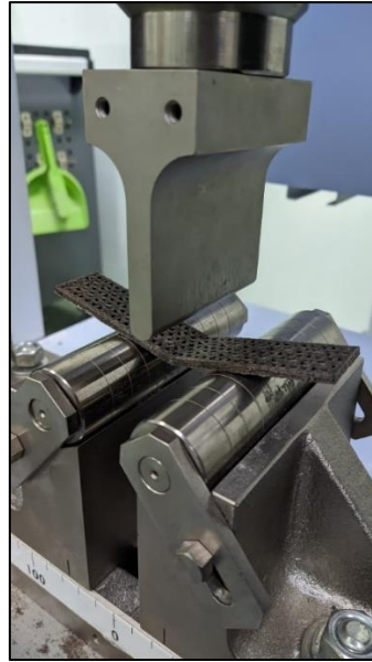
Figure 4.14 3-Point Bending Testing on sample
