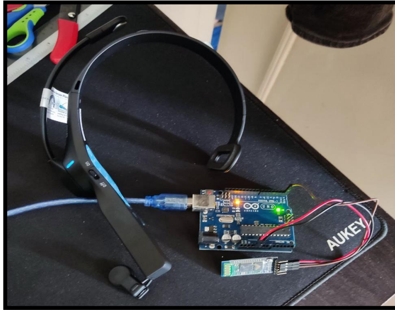
Figure 3.9 Neurosky Mindwave Mobile 2 successfully connected to HC-05
