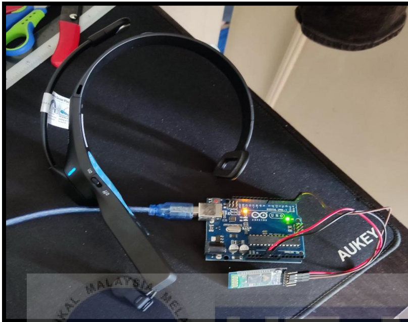
Figure 4.13 Neurosky Mindwave Mobile 2 headset connected to HC-05
