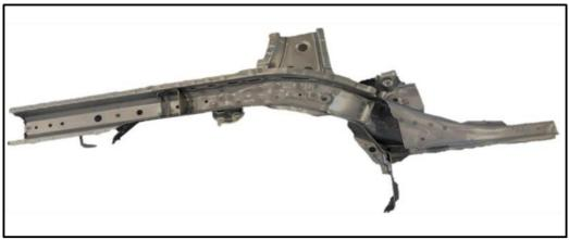
Figure 4.5 Frame Comp Rear LH (Left Hand)
