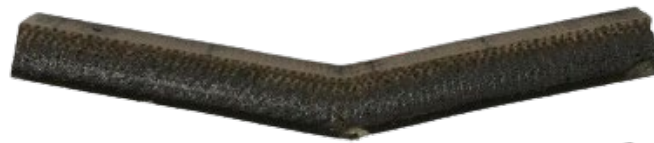
Figure 4.8 The failure mode of hybrid composite
