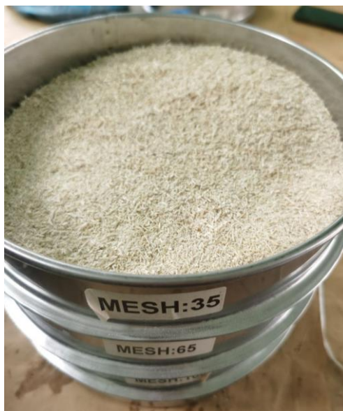
Figure 3.6 Mesh size of sugarcane bagasse is 35 mesh
