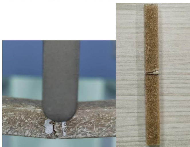
Figure 4.7 Result of flexural test
