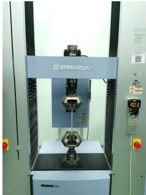
Figure 3.12 SHIMADZU universal testing machine (tensile test)
