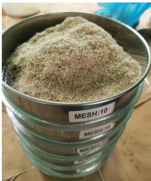
Figure 3.5 Sugarcane bagasse are poured on the top of sieve
