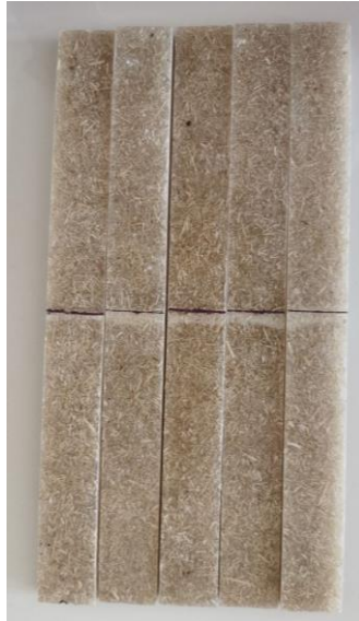
Figure 3.16 The centre of specimens have been marked as a guide
