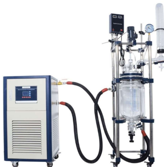
Figure 3.4 The Double Jacketed glass reactor integrated with heat circulator
