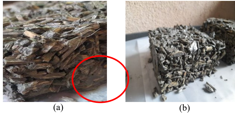
Figure 4.5 Selected sample after cured (a) cement with too much water (b) good samples that mix well
