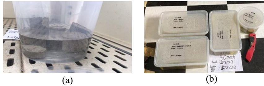
Figure 4.7 The curing process (a) at initial state a (b) at 28 days of submerging
