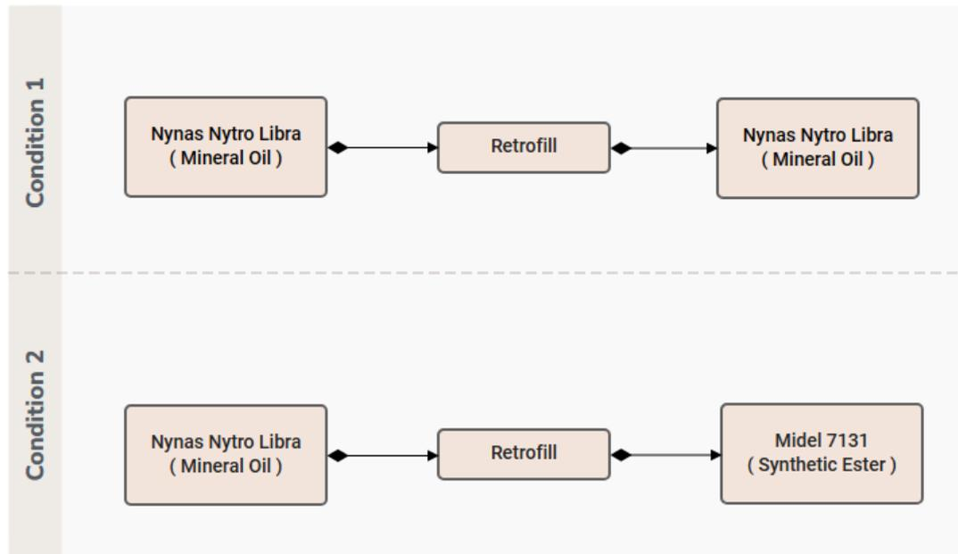
Figure 3–2: Retrofiling involving two conditions.
