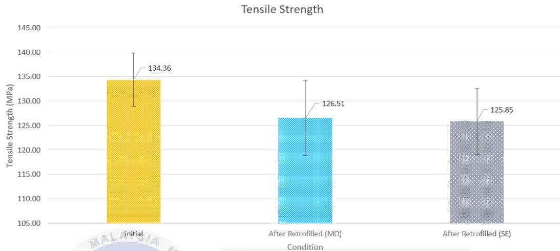
Figure 4–3: Tensile strength of kraft paper for initial and after retrofilled.
