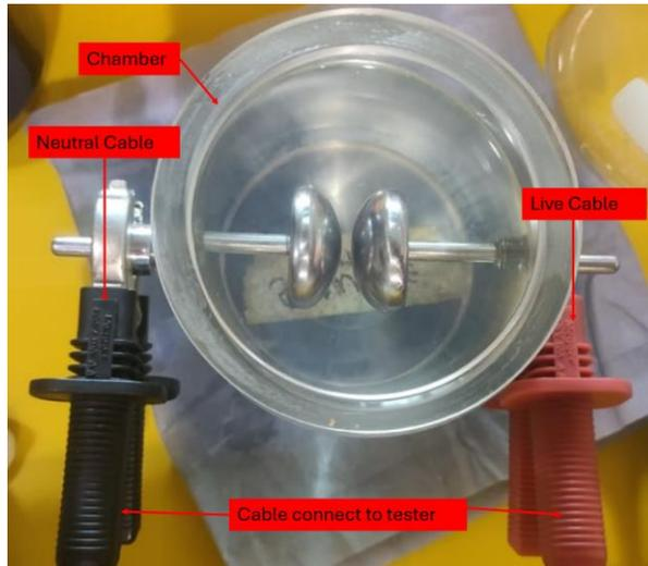
Figure 3–18: Chamber for polarization index testing.
