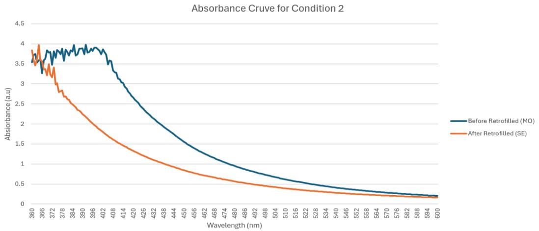
Figure 4–15: The absorbance characteristics of insulating oil (before and after retrofilled with SE) for condition 2.
