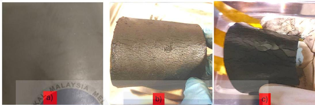
Figure 4–10: Comparison for condition of NBR gasket for a) initial and b) after retrofilled with MO and c) after retrofilled with SE.
