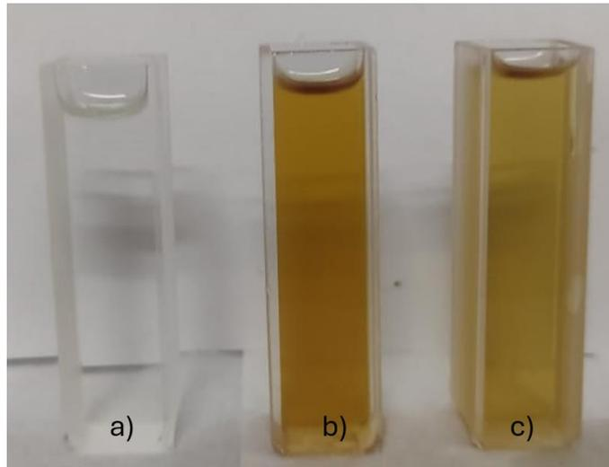
Figure 4-13: Color of insulating for Condition 2: a) MO before aging, b) MO before retrofilled and c) SE after retrofilled.
