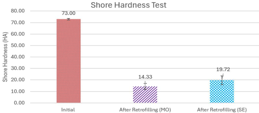
Figure 4–8: Shore hardness of the NBR gasket for a) initial, b) after retrofilled (MO) and c) after retrofilled (SE)
