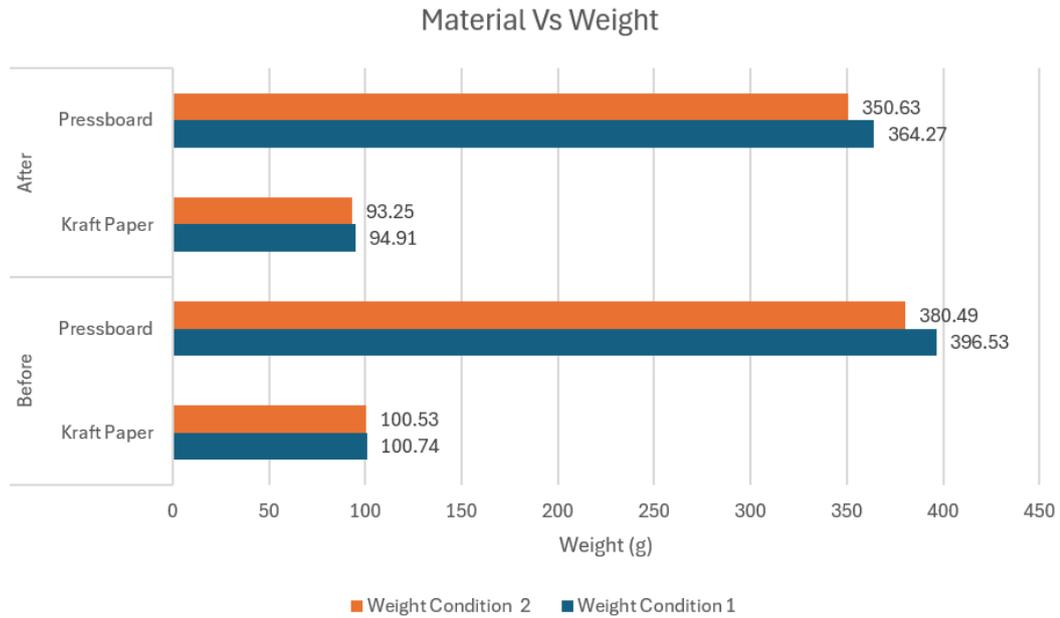
Figure 4–1: Graph for weight of kraft paper and pressboard before and after drying.
