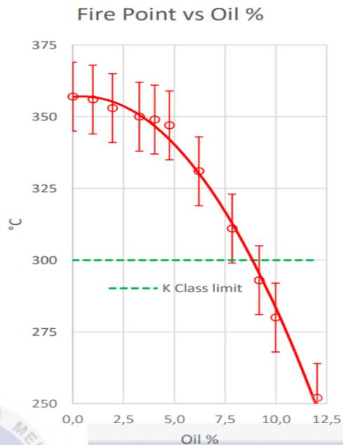
Figure 2–3: The effect of contamination on the fire point of insulating oil with error ( $\pm 13$  °C) [18].
