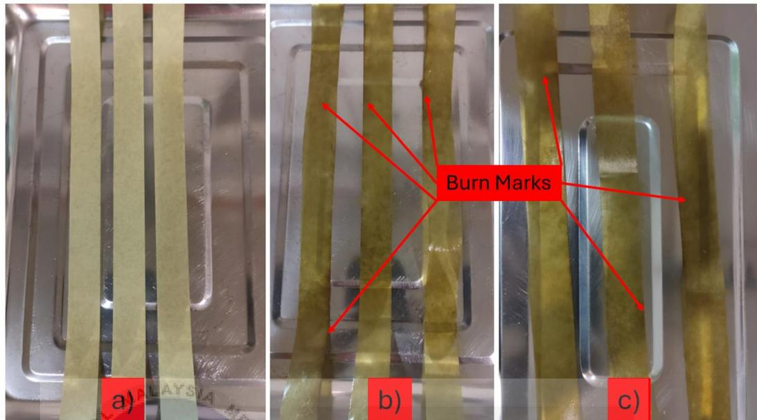
Figure 4–7: Comparison kraft paper a) initial condition, b) after retrofilled with MO and c) after retrofilled with SE.
