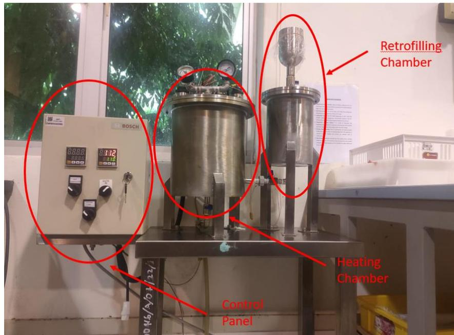
Figure 3-13 : Thermal aging tank.
