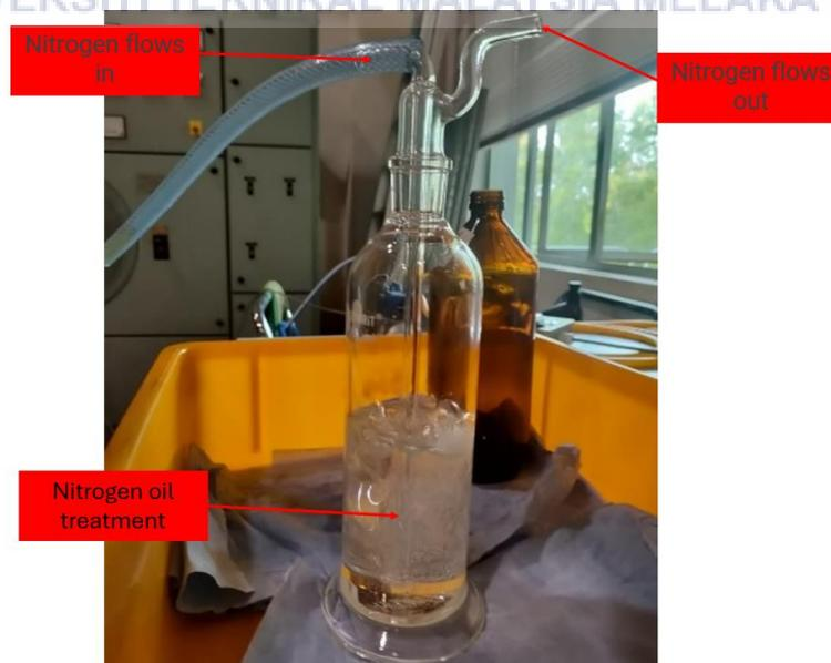
Figure 3–5: Nitrogen saturation process for oil sample.
