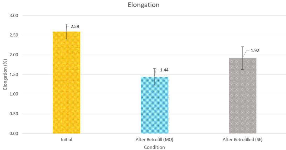
Figure 4–5: Elongation of kraft paper for initial and after retrofilled.
