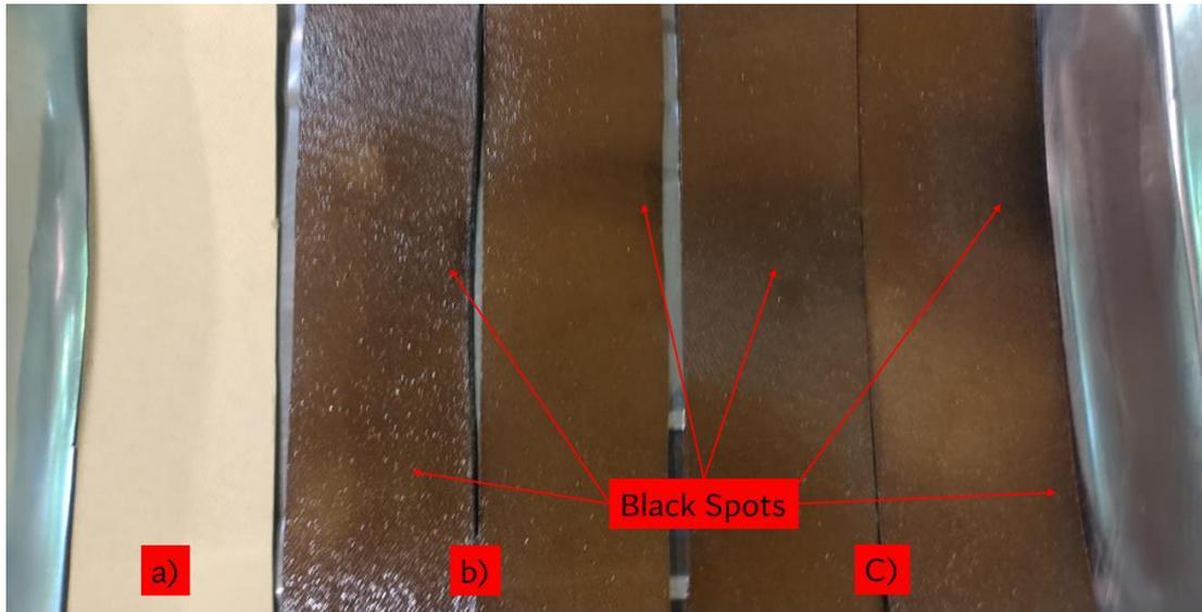
Figure 4–11: The color changes of the pressboard observed visually for a) initial, b) after retrofilled with MO and c) after retrofilled with SE.
