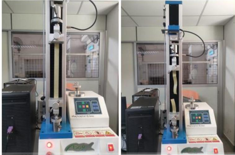
Figure 3–17: Tensile Test Machine.
