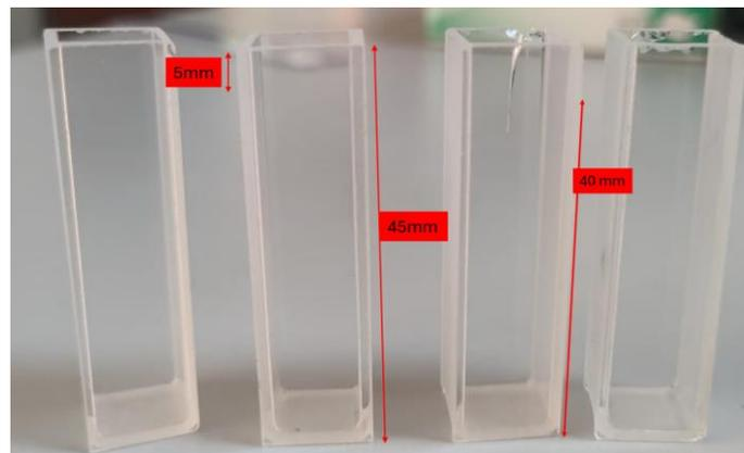
Figure 3–19: Measurement of cuvette height.
