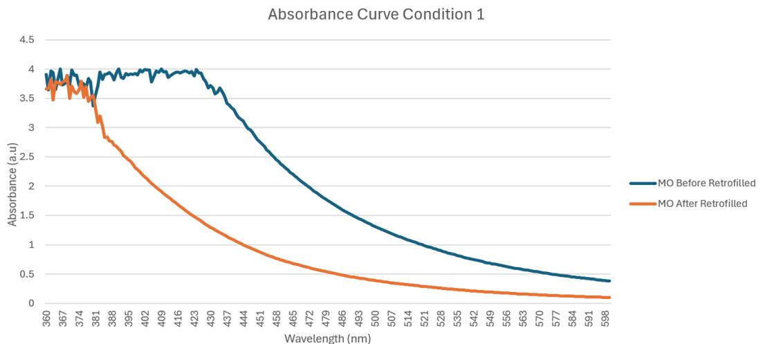
Figure 4-14: The absorbance characteristics of insulating oil (before and after retrofilled with MO) for condition 1.
