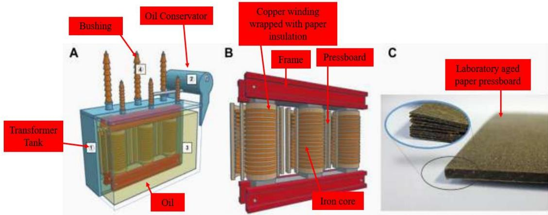
Figure 1–1: Show a) power transformer, b) power transformer core (section between core and winding and c) several kraft paper pressed by pressboard [4].
