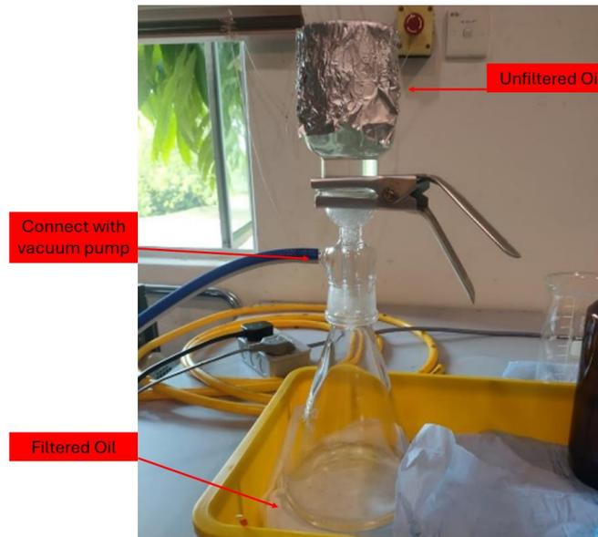
Figure 3–4: Process of filtering samples oil.
