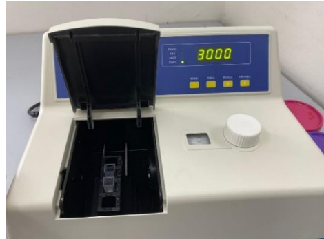
Figure 3.7 Curvettes (containing honey inside) are placed into the Spectrophotometer
