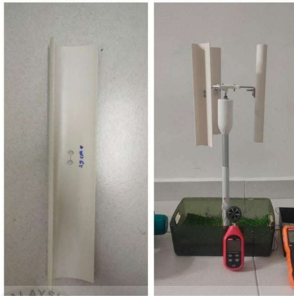
Figure 3.10 Show the VAWT being tested using UPVC as wind blade
