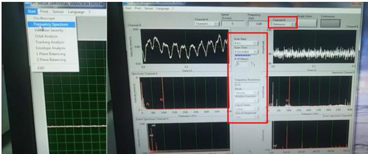
Figure 3.16 PT500.04 FFT Spectrum Settings
