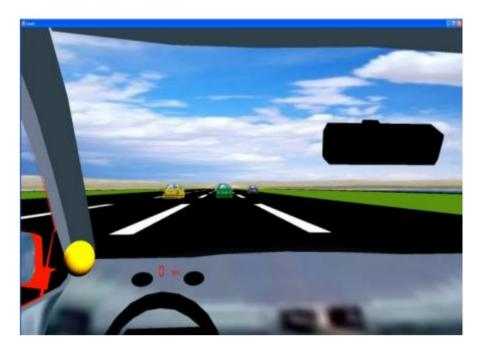
**Figure 2-29** - Screen shot of driving simulator. The driver interacts with the scene from within the driver's seat of the simulated vehicle. (Racine et al., 2010)
