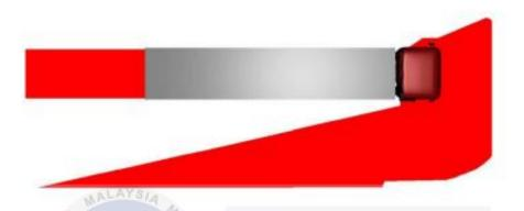
Figure 2-14 - Blind spot region (red) of the truck-trailer combination shown on the ground plane. The width is about 2 m. A large blind spot region arises in front of the vehicle as well as on the passenger's side.
