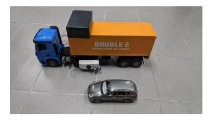
Figure 3-14 - Car In Truck blind spot
