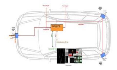
Figure 2-22 - Sensor Placement on a car
