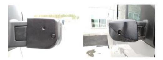
Figure 2-17 - Camera video attach at the bracket of side door
