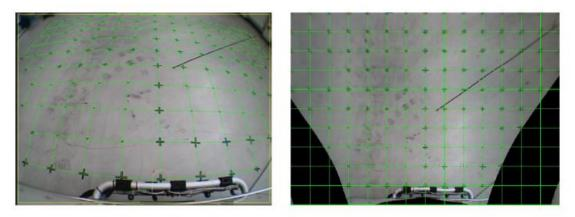
Figure 2-28 - Original and undistorted image of the grid
