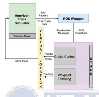
Figure 2-30 - American Truck Simulator Communication Flow (Darwesh et al., 2020)
