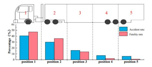
Figure 2-24 - Proportion and accident severity in each divided semitrailer truck
