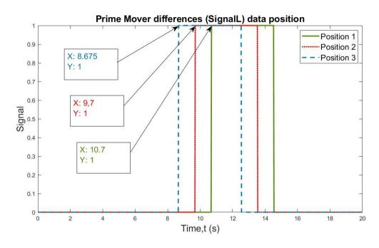
Figure 4-2 - Prime-mover sensor position signal graph
