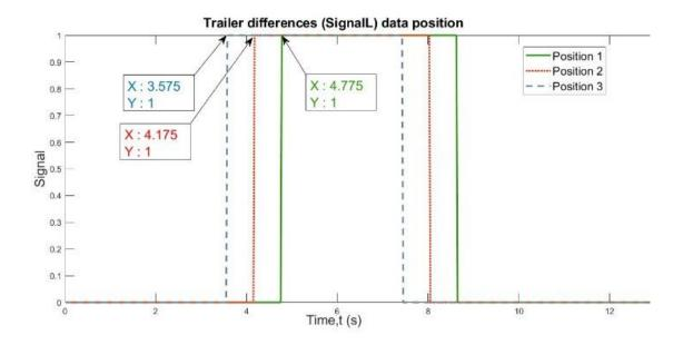
Figure 4-5 - Trailer sensor position signal graph
