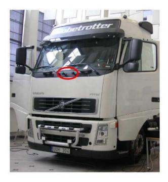
Figure 2-26 - Position for stero based vision blind spot detection system
