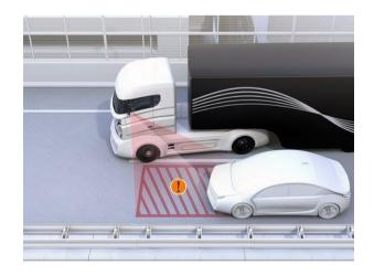
**Figure 2-11 - Side collision on blindspot region**
