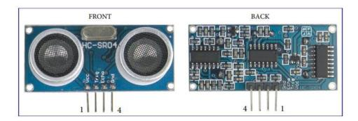
Figure 3-8 - Ultrasonic Sensor HC-SR04
