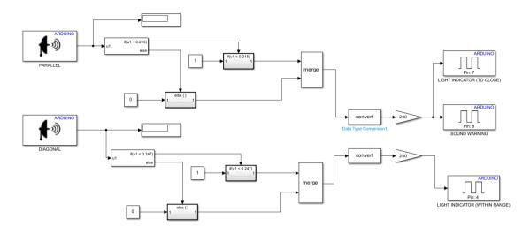
Figure 3-6 - Simulink Block Model for Sensor detection HIL
