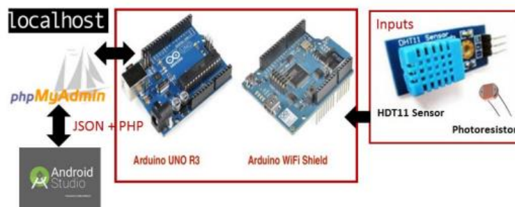
Figure 2.6 Temperature, humidity and light sensing for IoT system (Salha, 2017)
