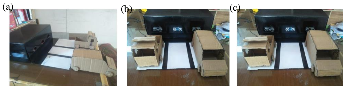
Figure 2.19 Ultrasonic sensor test at different distances. (a) 15 cm (b) 3 cm (c) 2 cm (Jenli,2021)
