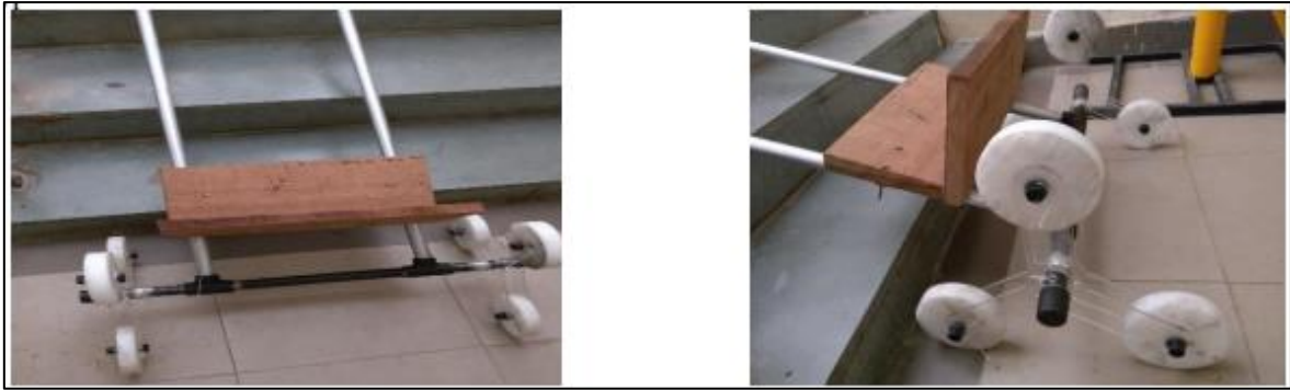
Figure 2.4 Tri-Wheel attachment concept on trolley (Ajay et al., 2017)
