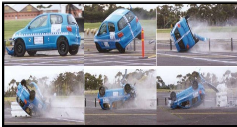
Figure 2-5 Vehicle motion during typical roll Bounce Over initiated rollover (Young et al., 2007)
