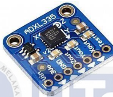
Figure 3:8 The accelerometer sensor (ADXL335-5V Ready Triple- Axis Accelerometer, n.d.)
