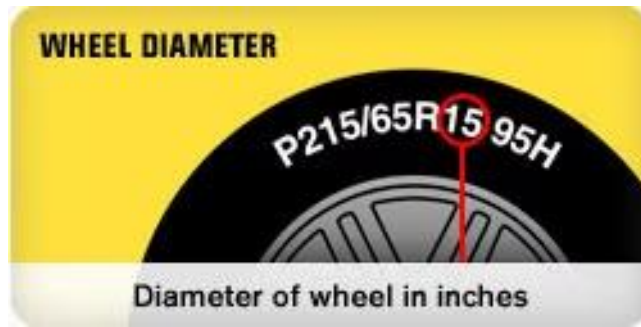
Figure 2.18 Shows Wheel Diameter of a Tire (Gent, 2006)
