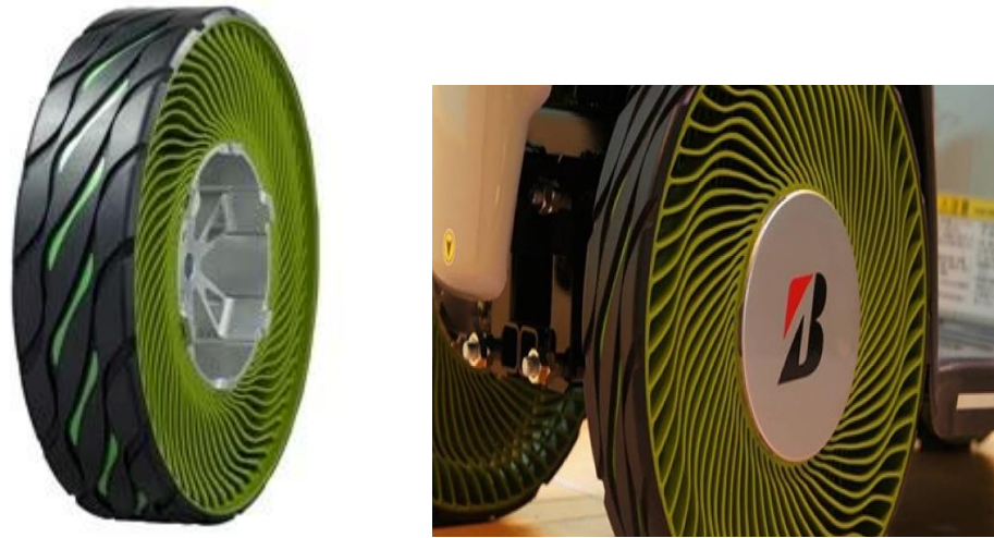
Figure 2.32 Show Bridgestone Second Generation Air-Free Airless Tire and Application in Gold Cart (Deng, Wang, Shen, Gong, & Xiao, 2022)
