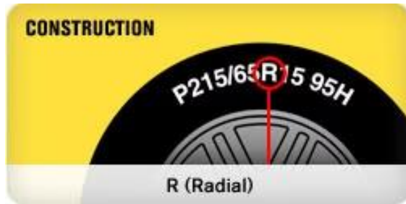
Figure 2.17 Shows Construction of a Tire (Gent, 2006)
