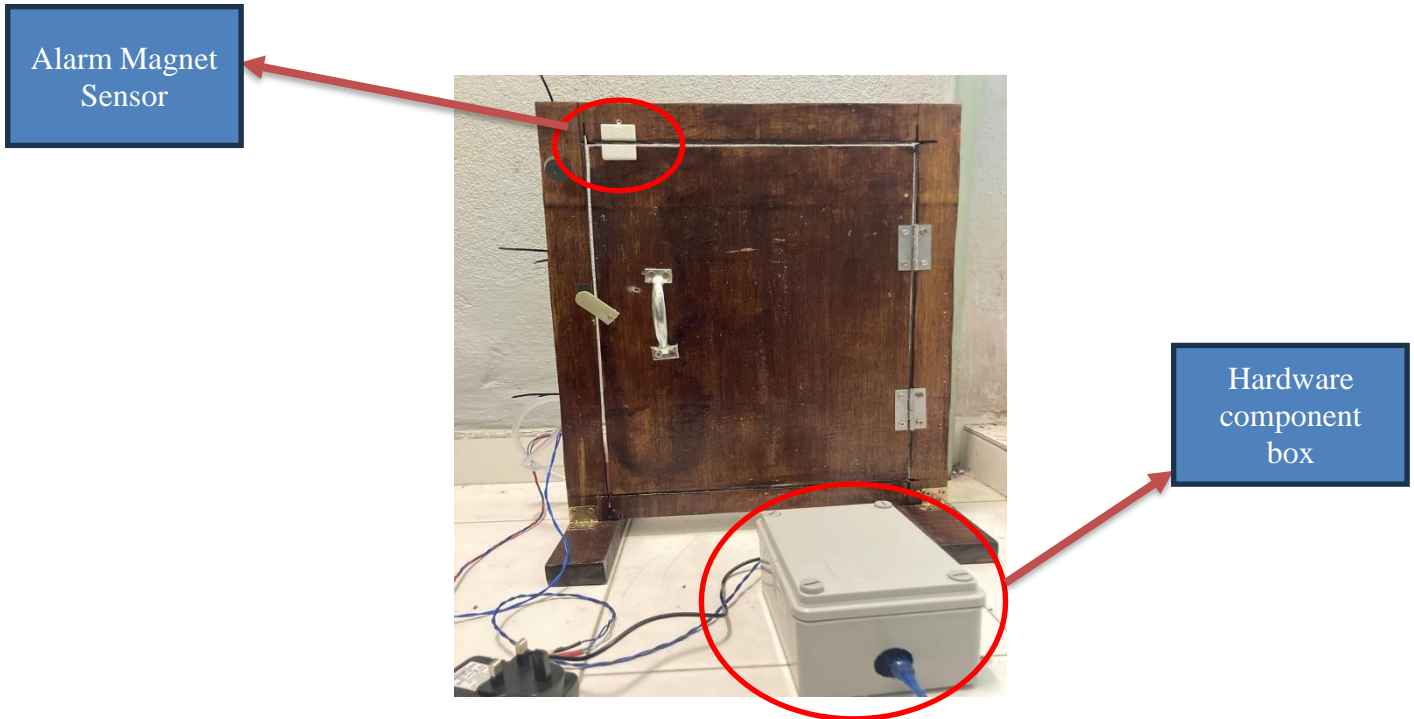
Figure 4.1: Smart Self-Hygiene Door system experimental setup
