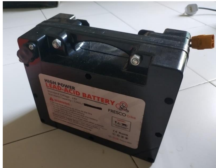
Figure 4.3.2.2 New 24 Volt Battery
