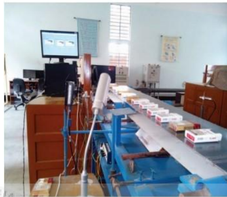
Figure 2.11: Experimental setup for product label quality control using image processing and classification techniques.
