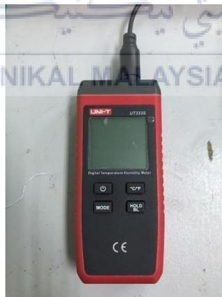
**Figure 2.9 Digital Humidity Temperature Meter**
