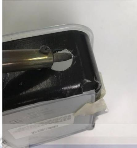
**Figure 3.10 Solder the container to make the hole.**
