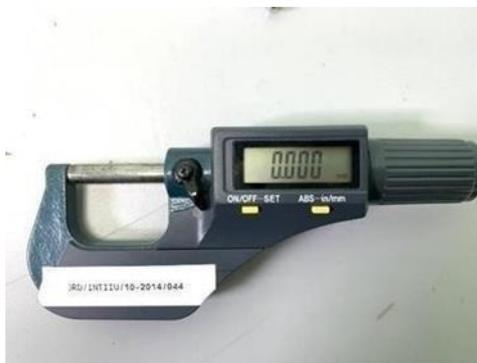
**Figure 3.7 Digital micrometer**
