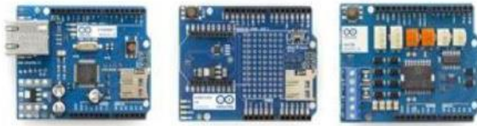
Figure 2-13 Arduino Shields – Ethernet, Wireless, Motor Driver
