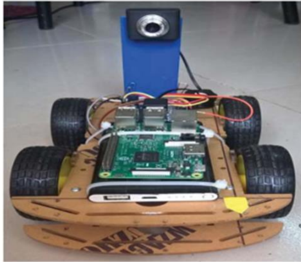
Figure 2.12: An 8 mega pixel webcam connected with the raspberry pi [18].
