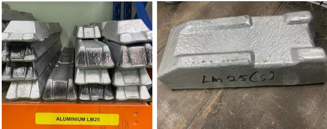
Figure 2.7: Ingot of Aluminium Alloy A356 /LM25.
