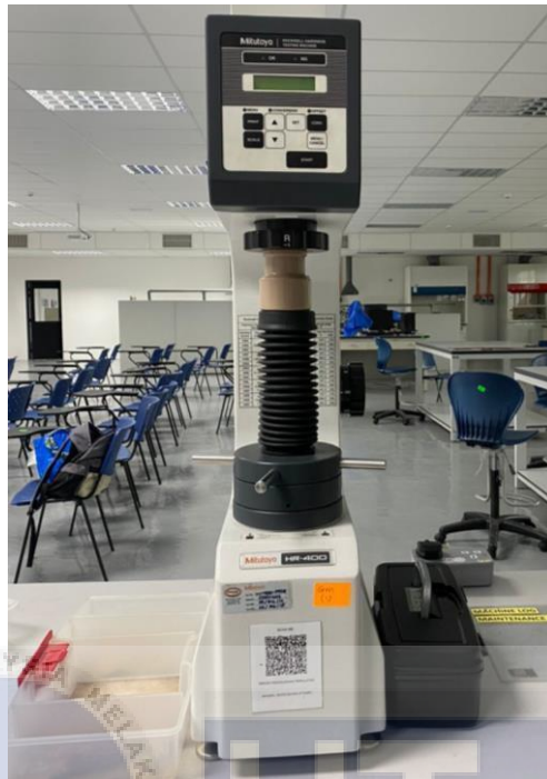
Figure 3.1: Rockwell hardness testing
