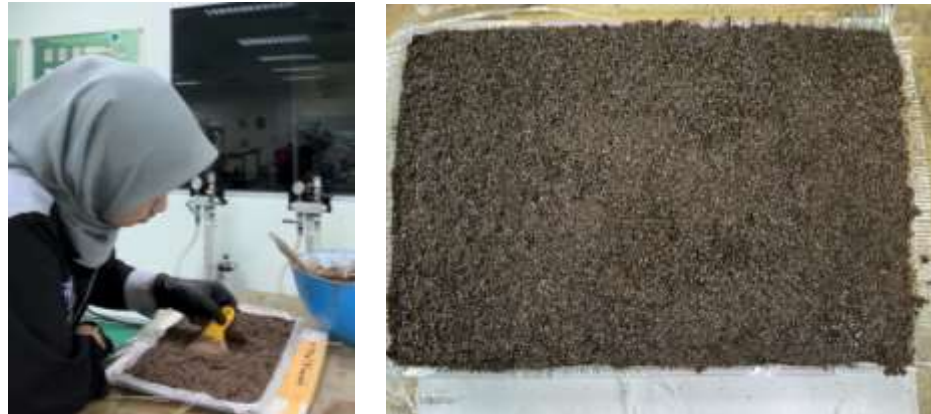
Figure 3.6 Hand layup process
