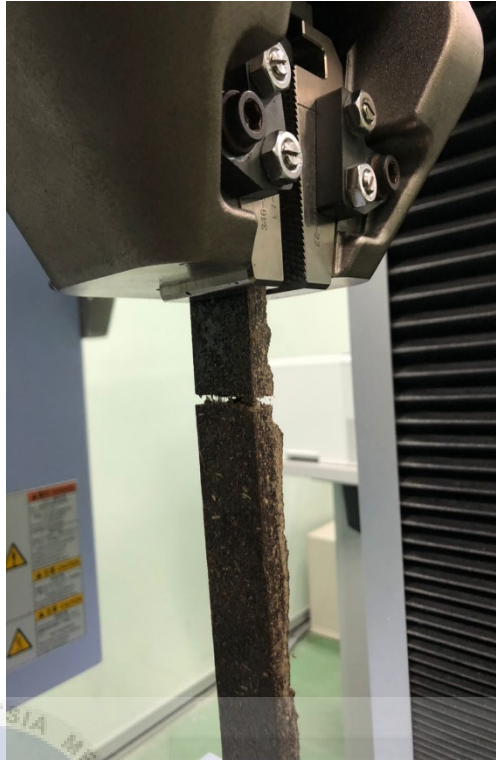
Figure 3.8.2 The specimen of a tensile test
