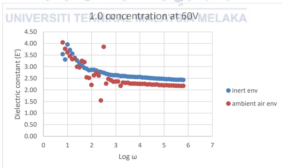
4.6 Graph dielectric constant ( $E'$ ) vs.  $\text{Log } \omega$  1.0mL concentration at 60V
