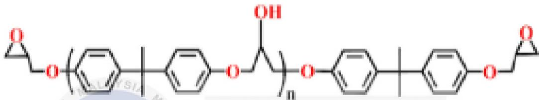
Figure 2.1 the chemical structure of a diglycidyl ether of bisphenol A (DGEBA)
