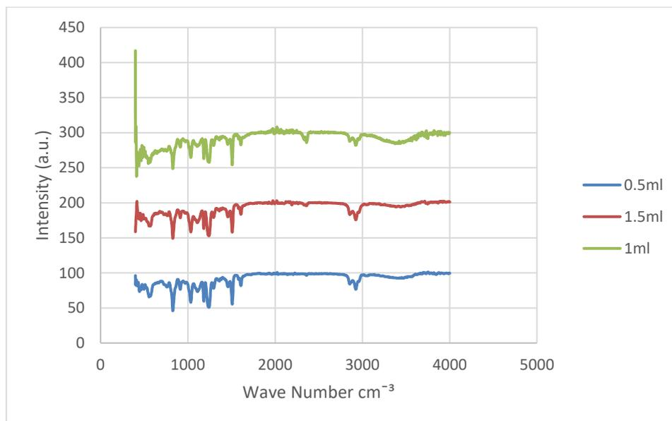
Figure 4.4 FTIR spectra of epoxy coating using solution produced in nitrogen gas environment.
