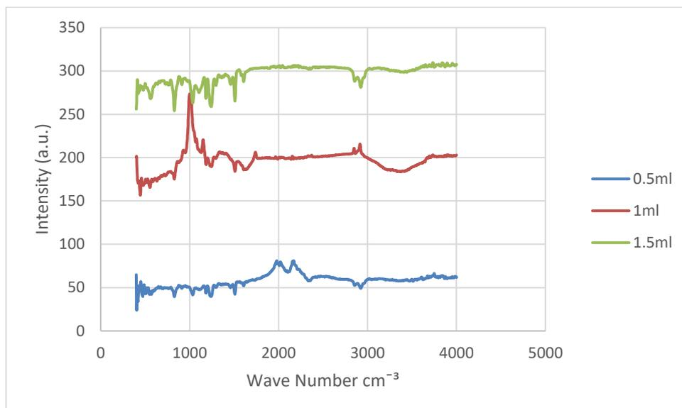
Figure 4.3 FTIR spectra of epoxy coating using solution produced in ambient air environment.
