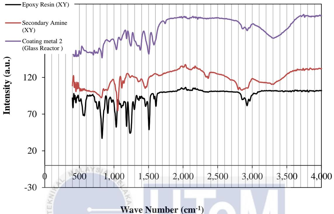
Figure 4.2 Combination FTIR graph of epoxy resin, secondary amine, and coating produce in ambient environment.
