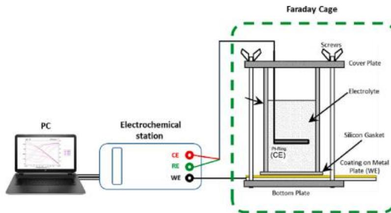
Figure 2.7 Schematic of the Electrochemical impedance spectroscopy (EIS) setup (Bakalli et al. 2023).
