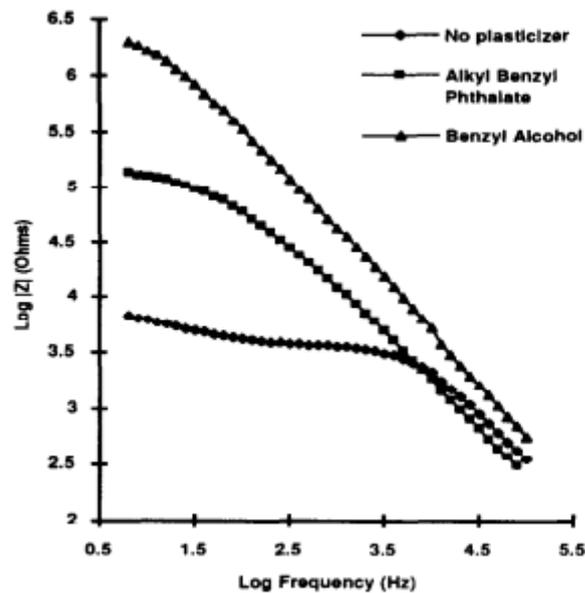
Figure 2.8 Example of Electrochemical impedance spectra (EIS) result (Mcintyre and Pham 1996).
