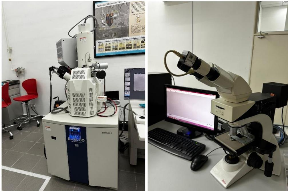
Figure 3.11 scanning electron microscope (SEM) and Optical Microscopy
