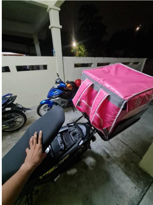
Figure 4.18 Opening the seat after pulling back the motorcycle rack fully
