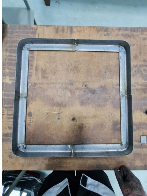
Figure 3.13 Joint and welded L shaped steel frames
