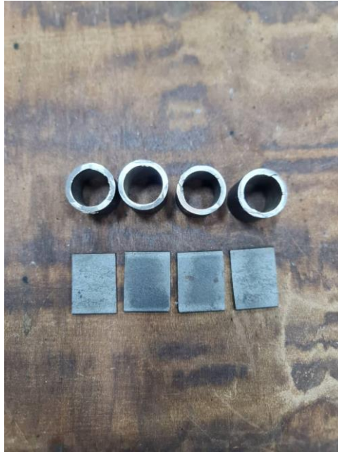
Figure 3.14 4 pieces of 0.5 cm thickness hollow steel pipe and 8 pieces of small plates
