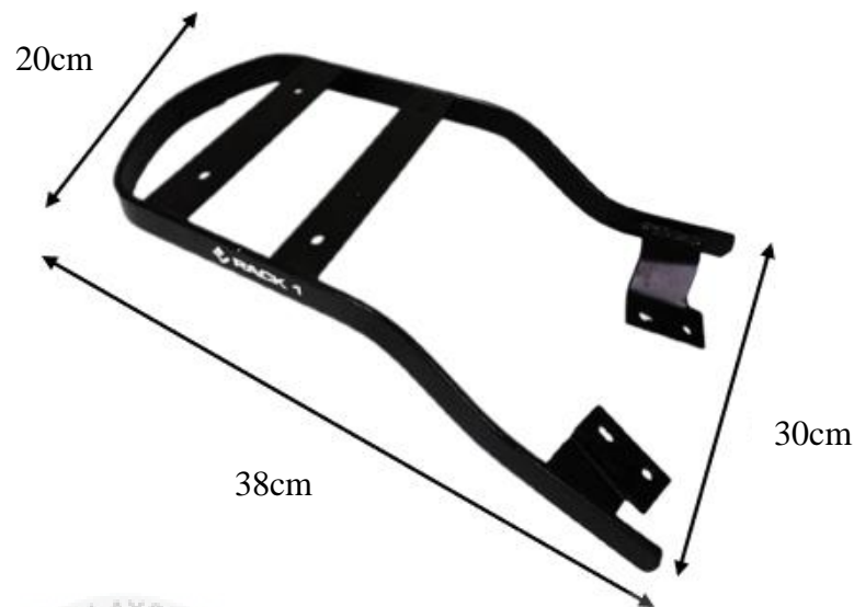
Figure 3.4 Rack holder dimensions for Y15ZR are 30cm(w) x 20cm(w) x 38cm(l)
