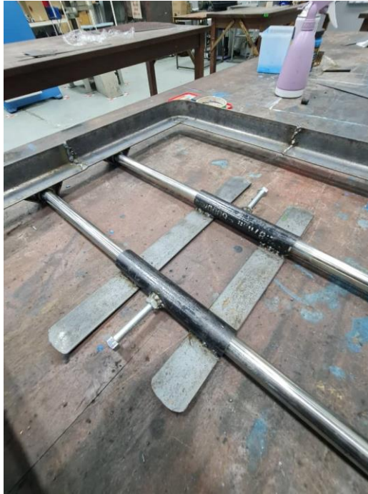
Figure 3.18 2 pieces 0.5 cm hollow steel pipe welded together with 2 steel plates
