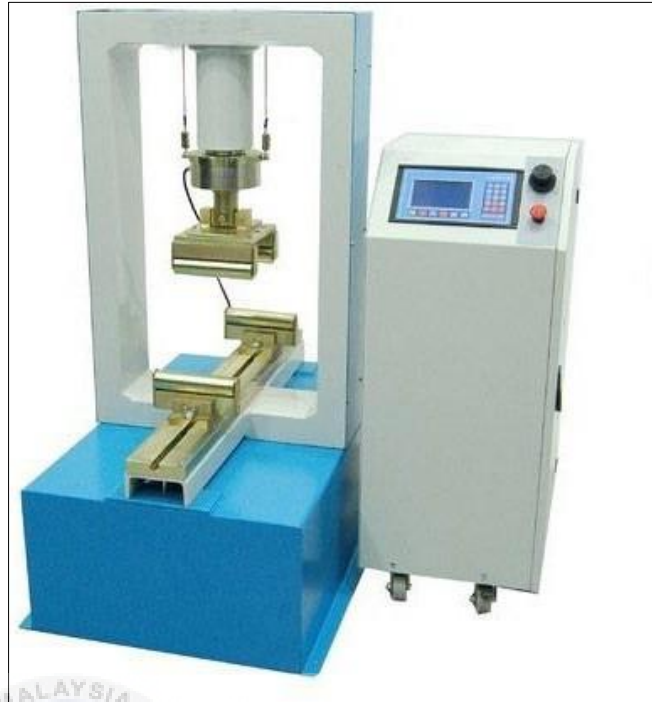
Figure 2.8: Example of flexural strength machine (Hamed et al., 2022)
