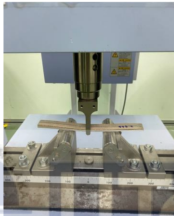
Figure 3.12: Specimen were placed horizontally in the three-point bend test
