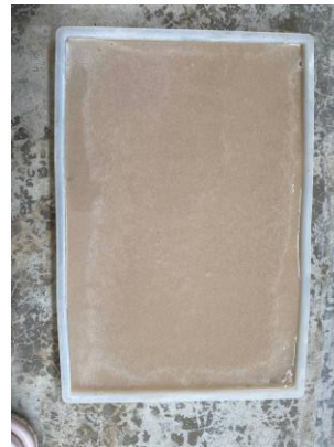
(f) Poured all mixture on top of jute
