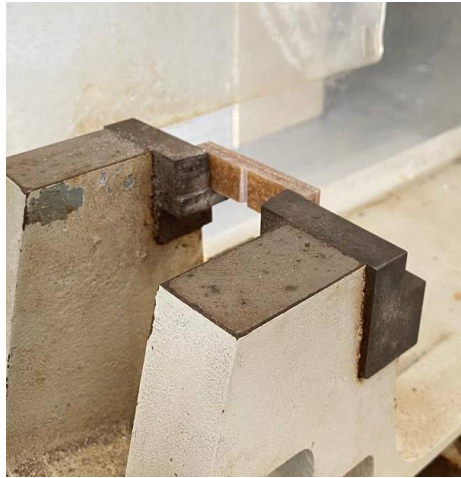
Figure 3.10: The impact test specimen struck and placed on an anvil
