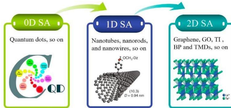
**Figure 2.3:** Classification of low-dimensional materials SA for fiber lasers.
