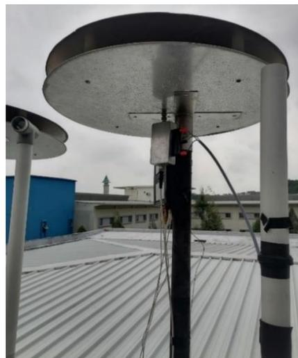
**Figure 3.15: Installation setup for Fast Field buffer circuit and antenna**
