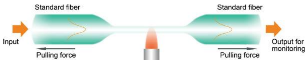
Figure 3.18 Microfiber Fabrication Technology with A Flame Heated Source
