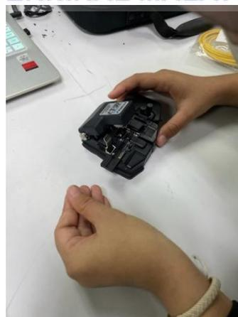
Figure 3.15 Cleaving process
