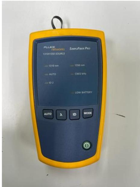
Figure 3.6 The light source that transmits 1310nm and 1550nm light
