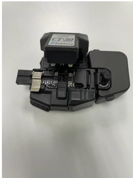
Figure 3.4 Hand cleaver used to cut the fibre tips to the proper length for splicing
