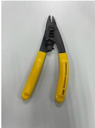
Figure 3.2 The jacket and cladding for the optical fibre cable are stripped away with a fibre cutter
