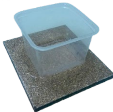
Figure 3. 13 : Water penetration test set-up
