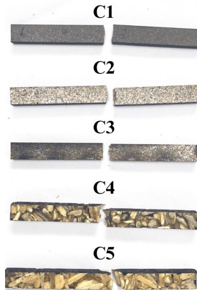
Figure 4. 4 The failure mode of kenaf core mix with polyester resin
