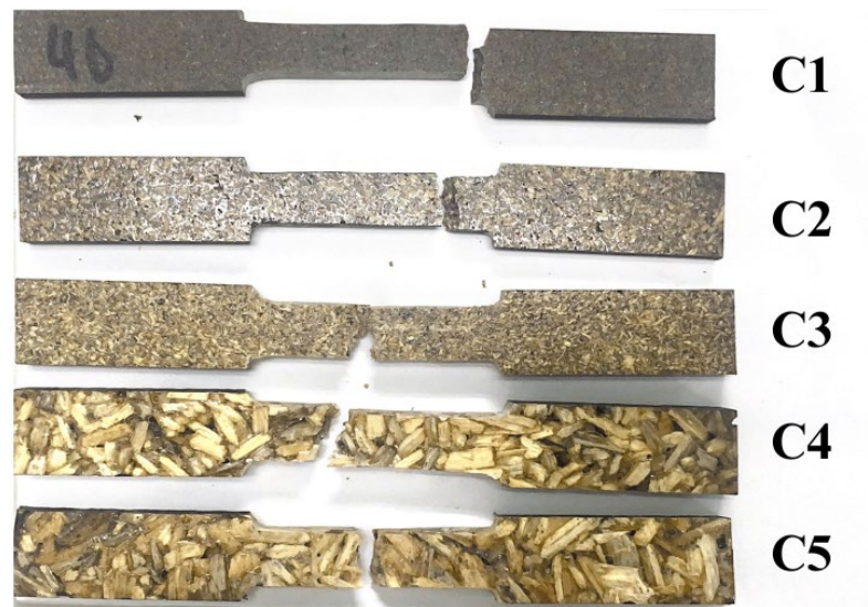
Figure 4. 2 The failure mode of kenaf core mix with polyester resin
