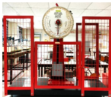
Figure 3. 11 : The Eurotech charpy impact tester
