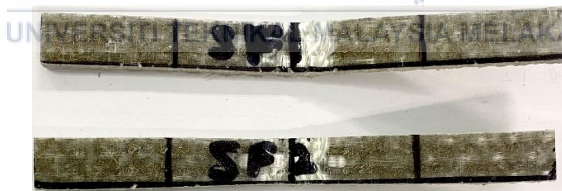
Figure 4.13 Sample for flexural testing in Phase 2
