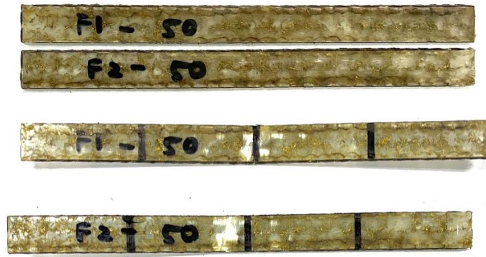
Figure 4.5 Sample for flexural testing in Phase 1.
