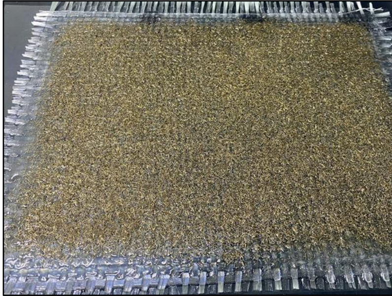
Figure 3.11 Placement of particulate wire waste.
