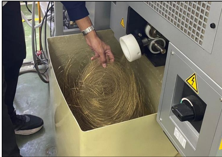
Figure 3.2 Scrap wire collection from the wire bin
