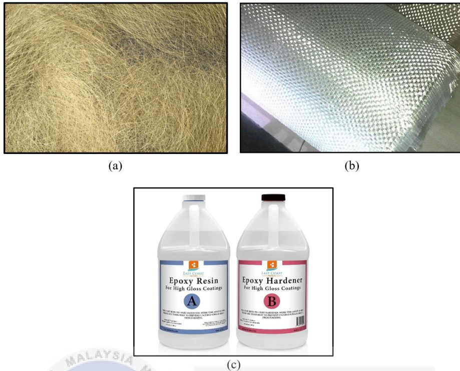
Figure 3.4 Raw materials for hand layup process (a) used brass wire; (b) fiberglass; (c) epoxy resin and hardener.
