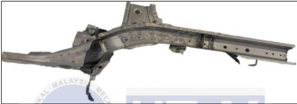
Figure 4.4 Final assembly of Frame Comp Rear RH
