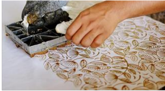
Figure 2.5: Making process of stamped batik [3]
