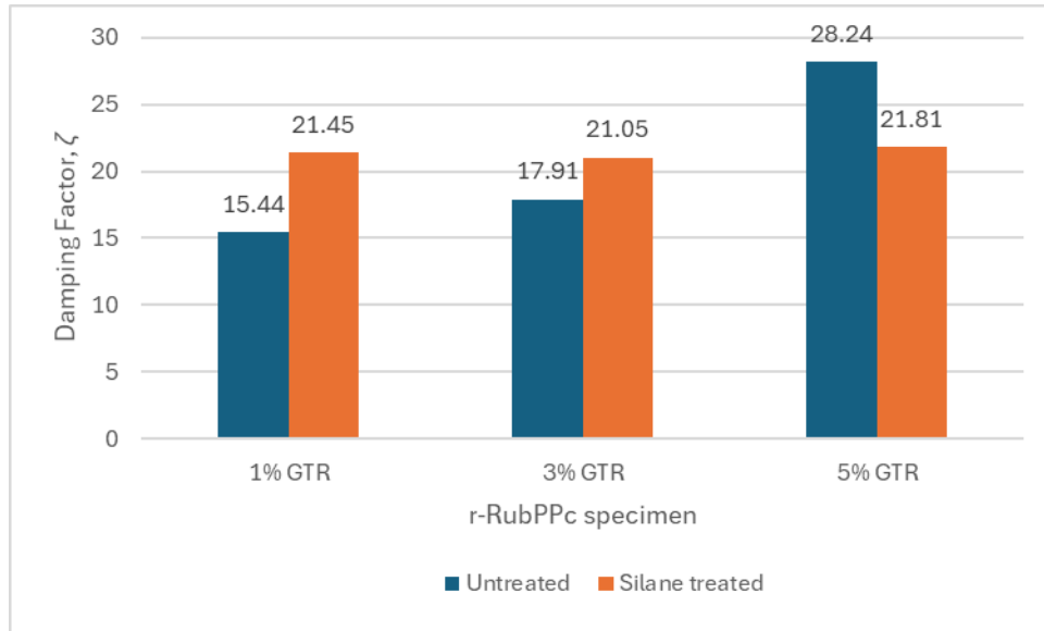
Figure 4.10 Damping factor, \zeta of r-RubPPc specimen
