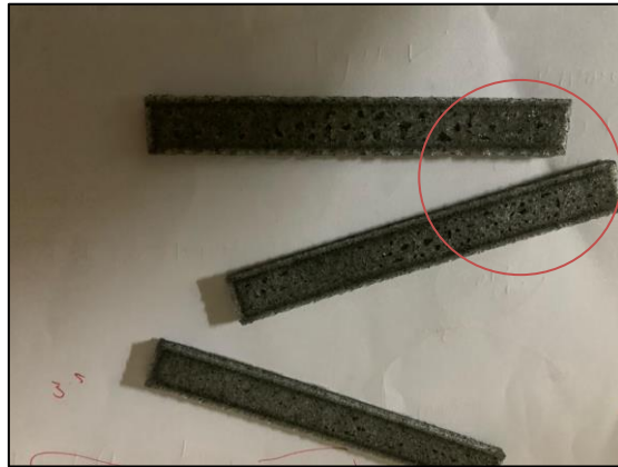
Figure 4.10 A less dense infill pattern comes decreased print quality and part success.
