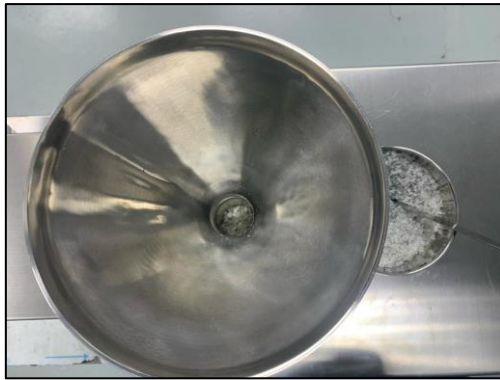
rPP/GTR pellet fed into the hopper
