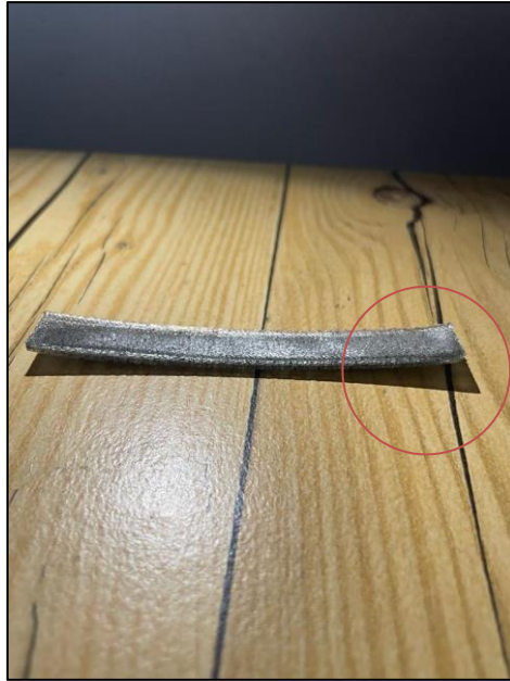
Figure 4.8 Sample rod for vibrational testing are warping
