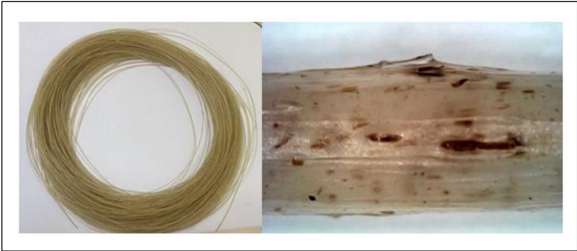
Figure 4.6 Filament & Microscope image of 3% MAPE
