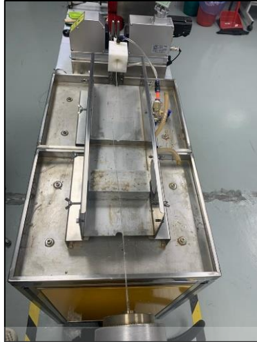
Figure 3.14 cooling water bath
