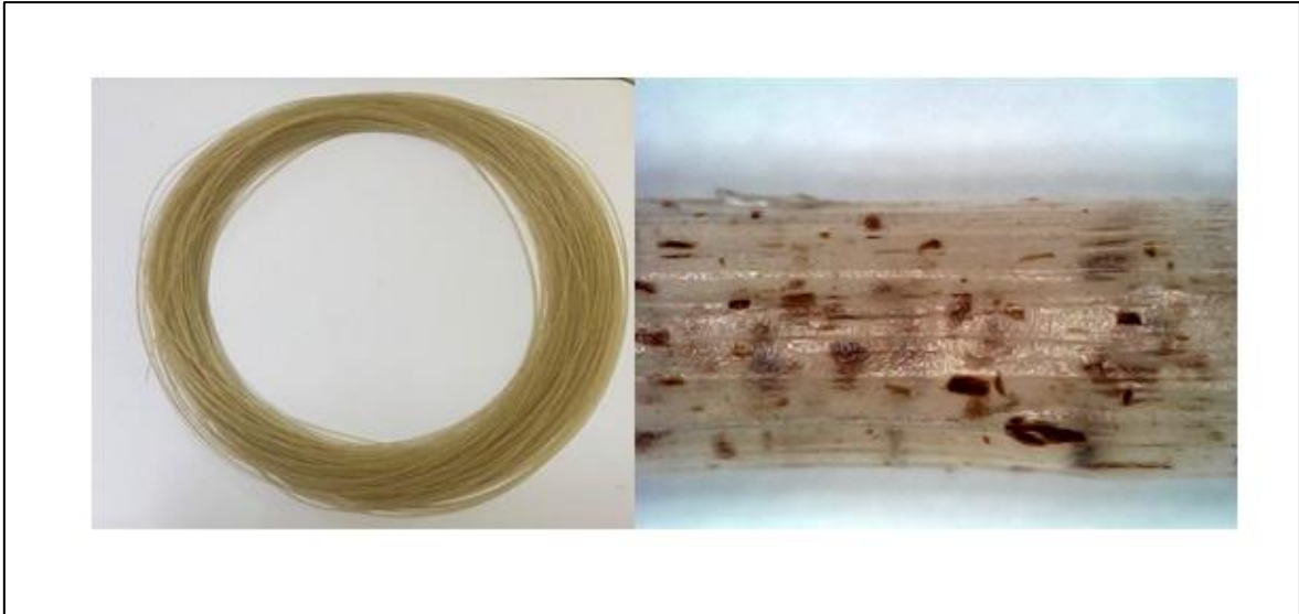
Figure 4.4 Filament & Microscope image of 0% MAPE
