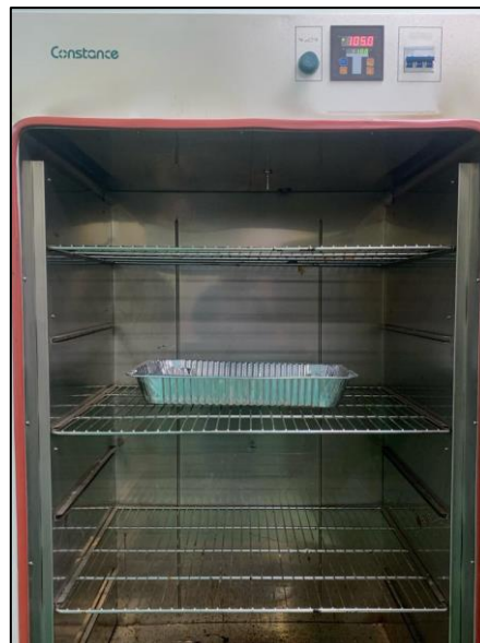
Figure 3.19 Oven used to Dried Specimen
