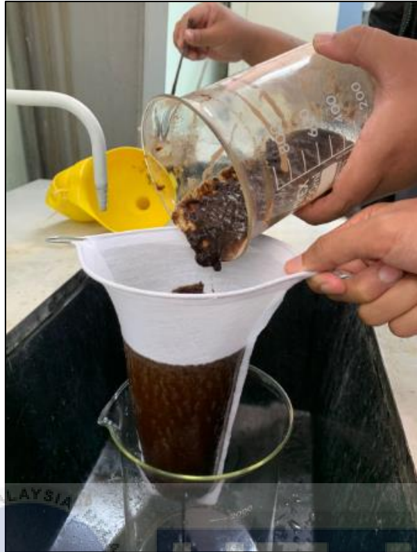
Figure 3.8 Cleaning Wood Fibre using Distilled Water
