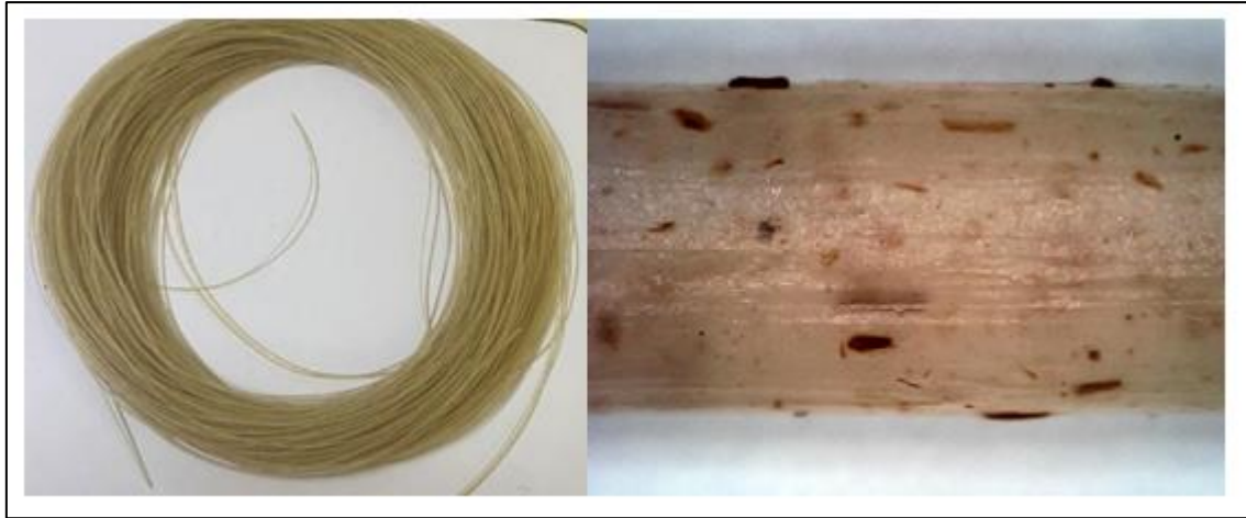
Figure 4.7 Filament & Microscope image of 5% MAPE
