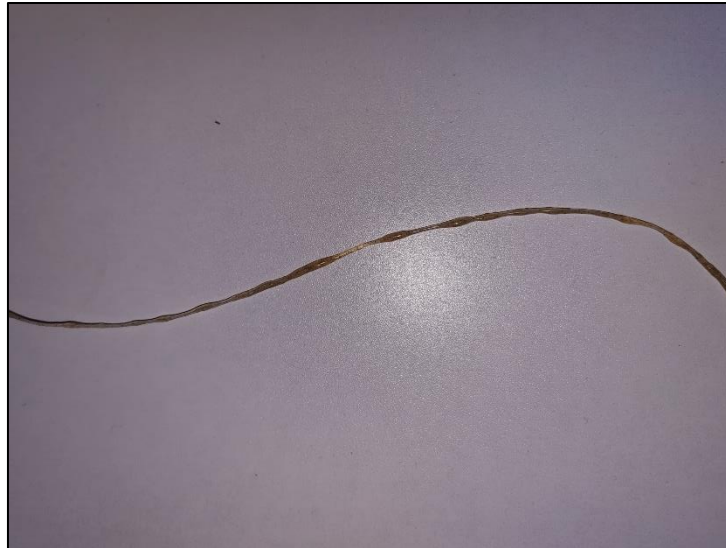
Figure 4.2 Sample filament sticky at entry hole cooling bath
